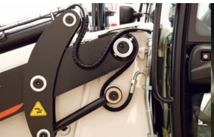
Recessed loader struts and aesthetic hose routing
