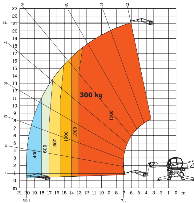
Rotation on extended stabilizers 3D positive / négative
