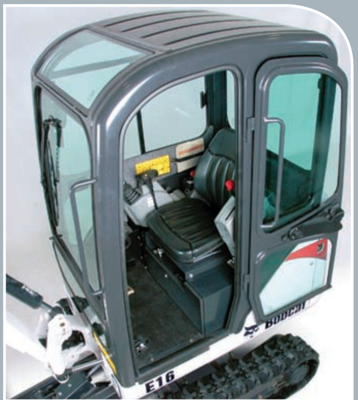
With a sturdy ROPS/TOPS canopy or cab and retractable seatbelt, you can focus on the job while feeling completely protected!
